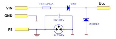
The electronic circuits of the IO module are galvanically separated from the PE, which is connected to the GND by a lightning arrester. The PE and GND department enables reliable operation of the system even in applications with differences in ground potentials.
