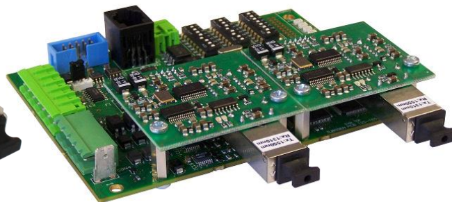
Modules installed on the control panel network board
